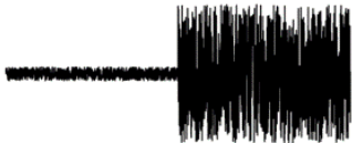
FIG. 3. The stimulus was a white-noise velocity signal modulated by a square wave envelope that switches between two values, \sigma_1 and \sigma_2 , with some period T . Source:[3]
